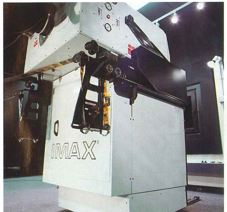
The IMAX GT 3D projector is bigger than a Mini and houses ten mirrors and two 15,000W lamps.
