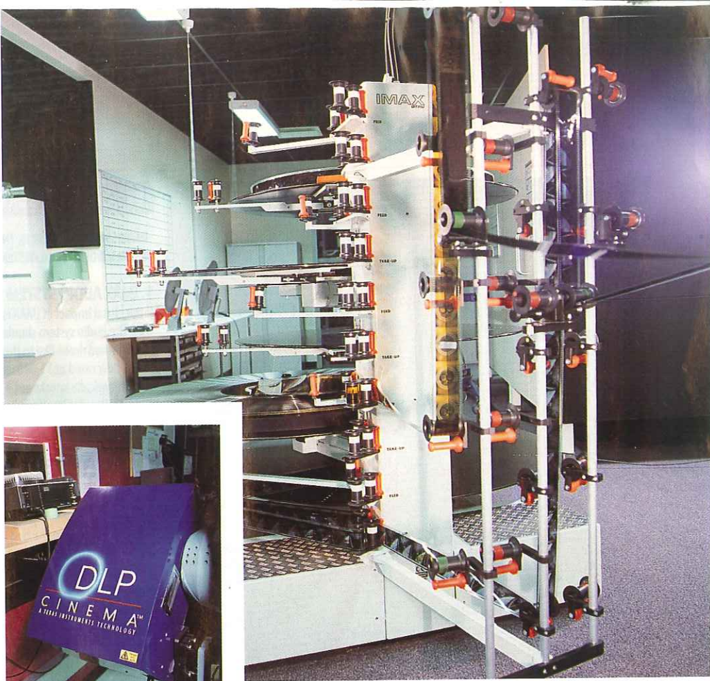
Above: The platter for the IMAX system, which transports the film to and from the projector. Left: The Texas Instruments Digital Light Processor head.
